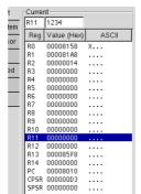
Modifying the contents of memory is slightly trickier. First, enter the appropriate address in the **Address** edit field and press ENTER. That address will now be displayed.<sup>4</sup> Next, use the TAB key to move to the **Hex** field (next to the **Address** field), then use the BACKSPACE and arrow keys as appropriate to delete any value there. Finally, you can enter the new value as a hexadecimal number, with or without the 0x prefix:
