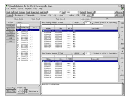
If it does not, check that the DSLMU Microcontroller Board is turned on and is ready, that the serial cable is firmly plugged in, and try again. If it still does not work, try replacing **kmd** with **kmd** -v to get some low-level debugging messages that might help diagnose the problem.
